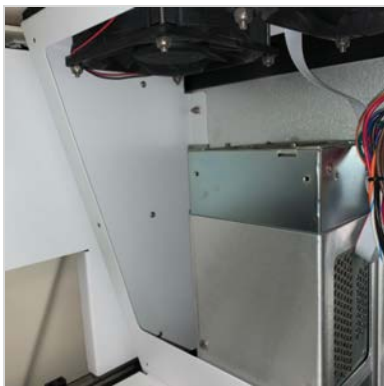
Fig: Three hidden screws for the left side panel
