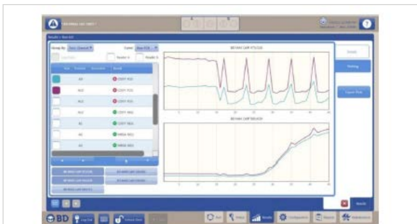
Plot 1: False Positive due to saw-tooth raw signal in Raw PCR mode
