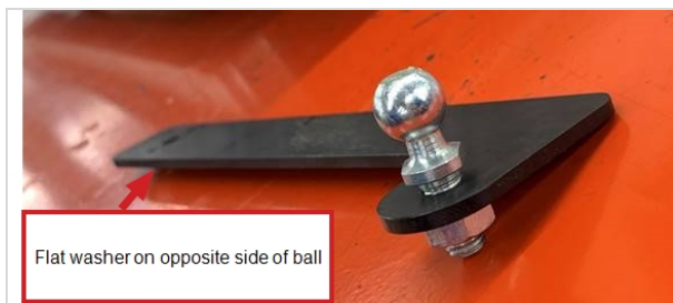
Fig: Ball joint installed in arm damper. Hand tighten all the way
