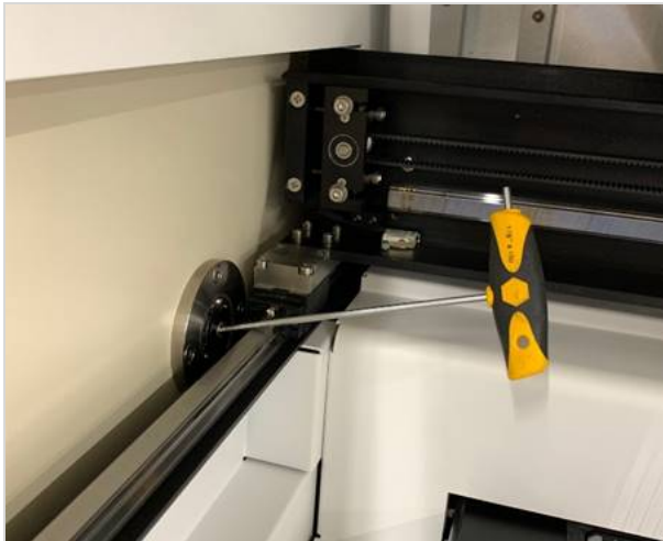
Fig: Ball-end Allen wrench needed to remove left side screw and retaining washer (black)
