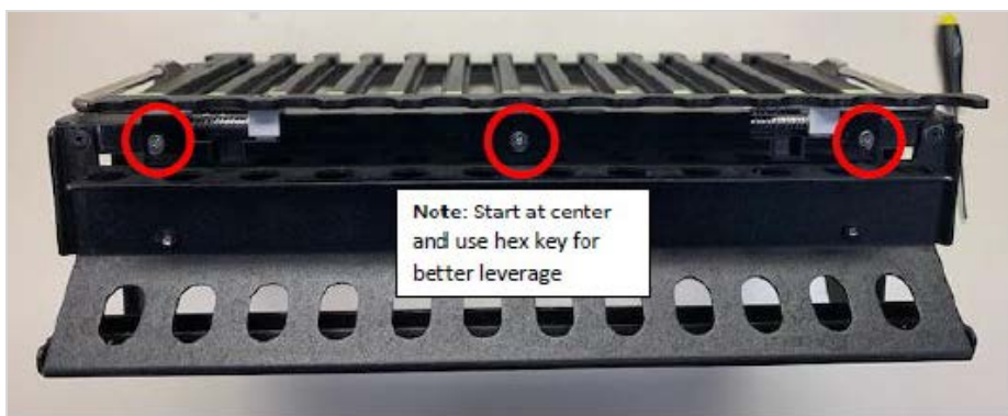
Fig: Front of current rack configuration showing screws to be replaced using the hex tool or screwdriver in the rack upgrade kit.
