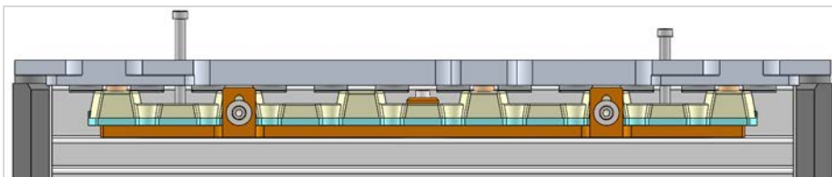
Fig: Fixed Magnet Assembly adhered to the mag/lysis assembly, side view
