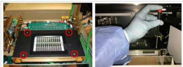
Fig: Location of the four screws holding the splash guard
