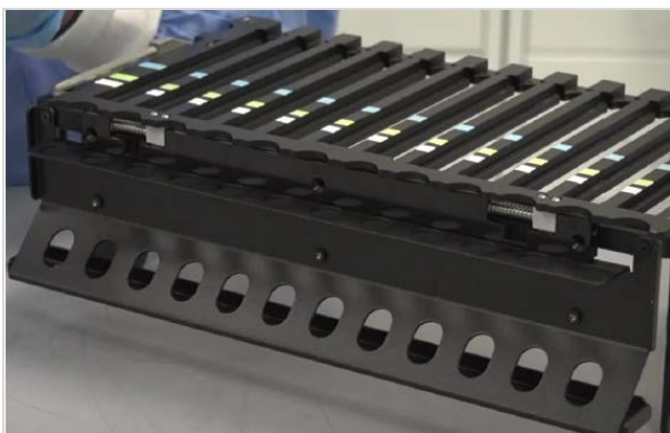
Fig: Front view of the rack with the slide locking mechanism in place.
