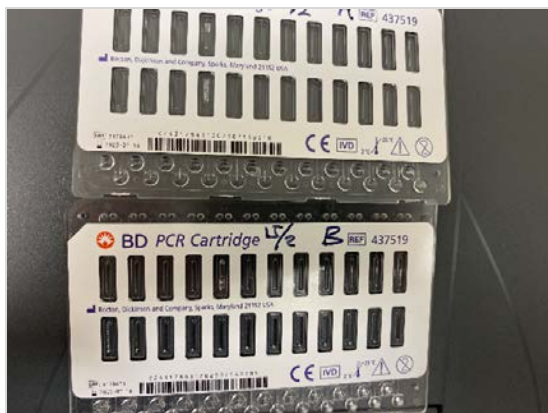
Figure 18: Cartridge example after the run showing both good and bad (bubbles) fills.
