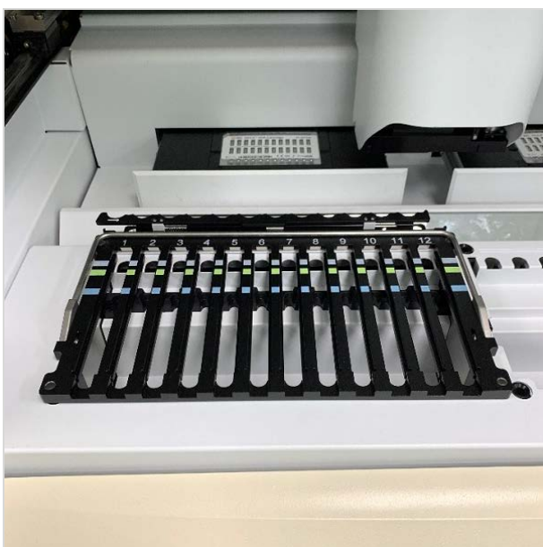
Fig: BD MAX Sample Rack loaded above new Fixed Magnet Assembly version 2
