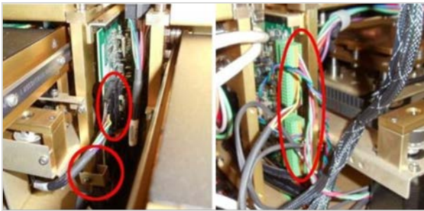
Fig: Disconnection points of cables on the Liberty board and 2X Motor Drive Max6 board.
