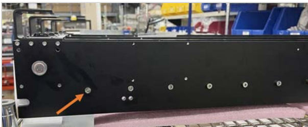
Fig: Right side fastener (bank 6) for newer systems
