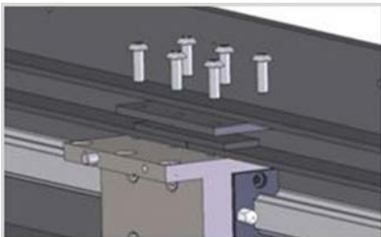
Fig: Tension is adjusted at the idler assembly.
