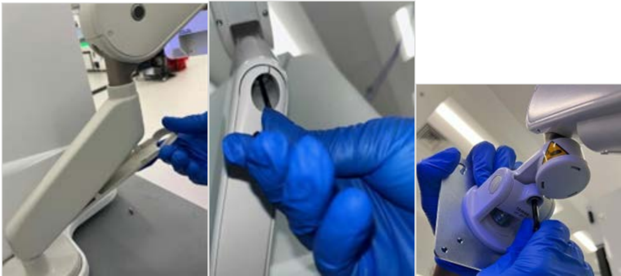
Figure 10: Cable duct (left) and two tension screws in the “elbow” (middle) and “wrist” (right).
