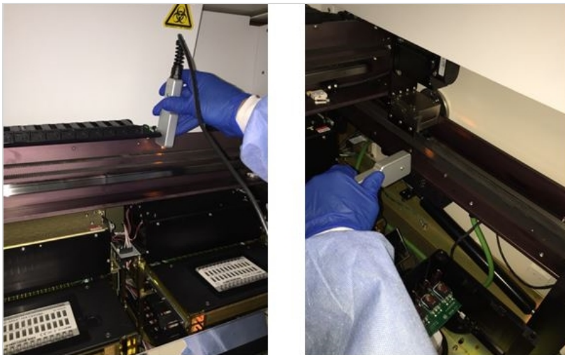
Fig: Checking X-Gantry belt tension (left) and Y-Gantry belt tension (right)
