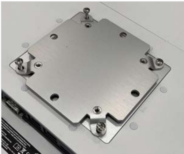
Figure 6: VESA mount on back of AIO
