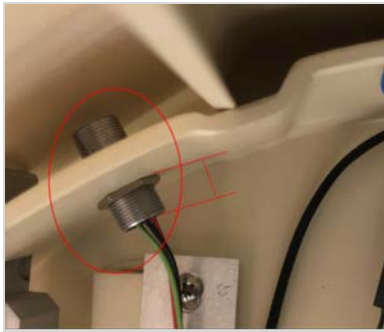
Fig: The lower part of the sensor should protrude about 0.45in to ensure the outer portion is the right distance from the door.
