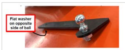
Fig: Ball joint installed in arm damper. Hand tighten all the way.
